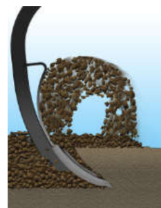
Point with ridge, same depth, reduced mixing.
